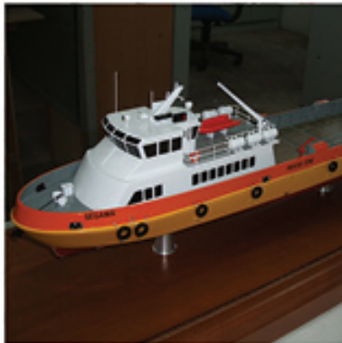
Project : 40-Man Utility Crew Boat, 30 knots triple Screw 5000 Hp Aluminum Vessel to ABS-HSC class
